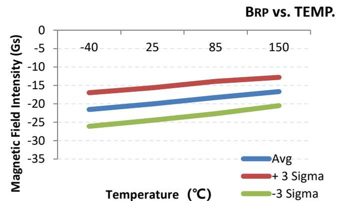
Figure.5 Magnetic Characteristics (BOP & BRP) vs. Temperature @  $V_{DD} = 5V$
