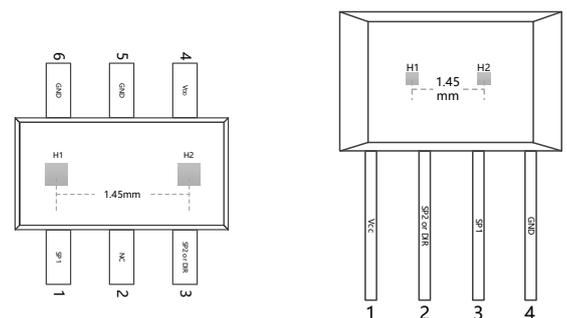
**Figure.1** Pin Configuration & Functions
