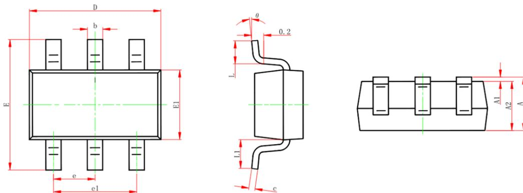
Figure.15 SOT-23-6L Package Drawing
